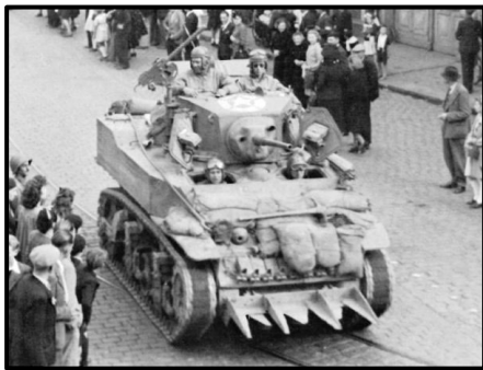
Notice welded “teeth” used to break through the hedgerows of France.
